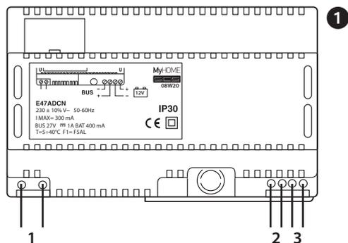
Connect the 230V a.c. power supply wires to the terminals (1) and the telephone pair to the terminals (2).
