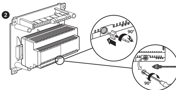
Extract the protection device completely.
