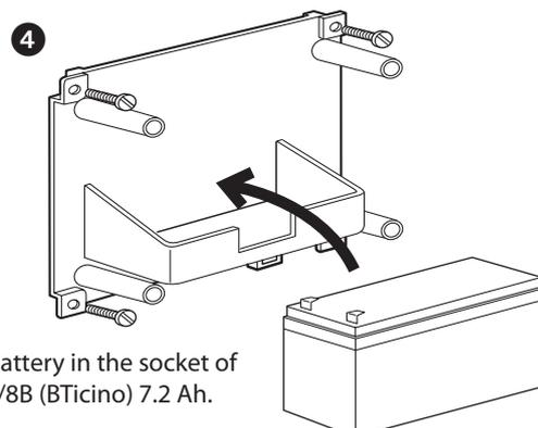
Install the back-up battery in the socket of container item F115/8B (BTicino) 7.2 Ah.
