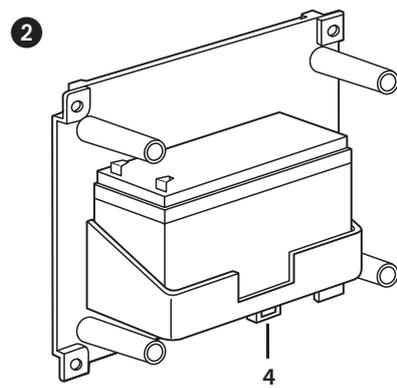
If you want to protect the battery compartment, connect the contact on the container item F115/8B (BTicino) (4) to a tamper line.
