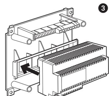
Install the power supply inside the switchboard item F115/8A (BTicino)
