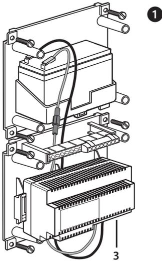
Connect the batteries to the power supply terminals (3) using the correct wire complete with protection with fuse.
