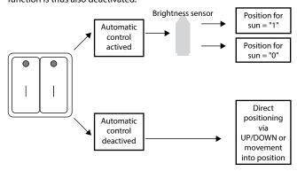
The Shutter actuator receives the information via the brightness sensor as to whether there is direct sunlight on the window. Once the delay period has elapsed, the Shutter actuator positions the shutter/blind according to the set Position for sun="1" (sun) or Position for sun="0" (no sun).
