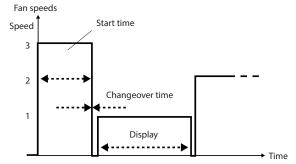
Fig. 6.8 Fan gear shifting mode
