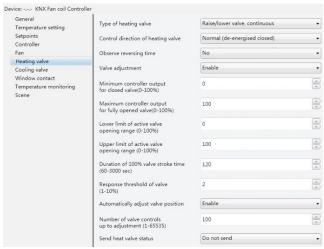
Fig. 6.9 "Heating valve" Parameter setting interface
