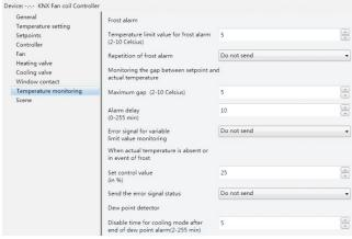
Fig.6.11 Parameter setting window of "Temperature monitoring"
