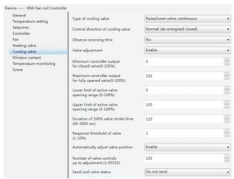
Fig. 6.9 "Cooling valve" Parameter setting interface
