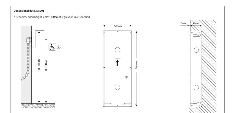
To ensure proper operation, the Fingerprint Reader must be installed in a location protected from rain.
