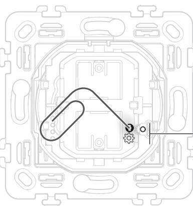
**3** Press and hold down the reset pushbutton until it flashes red. Now release. The reset has been done.
