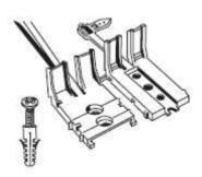
Adjusting the support according to the size of the cover
