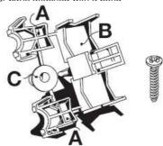
Adjusting the support according to the diameters (ranging from 10 to  $22\mathrm{mm}$ )
