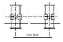
It is recommended that pipe clips are fitted every 50cm to ensure alignment
