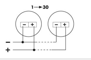
9 V battery operation Note: Interconnection with max. 30 detectors, max. line length 300 m.
