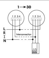
Connection 230 V AC and interconnection + external switching relay (optional) for switching of external devices such as sirens, flashlights and telephone diallers.
