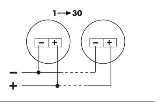
9 V battery operation Note: Interconnection with max. 30 detectors, max. line length 300 m.
