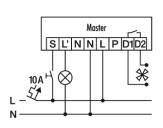
Standard operation with additional control by means of a closing button. If required, the light can be manually switched on or off with the button.
