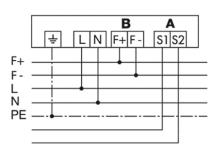
(A) Fail-safe contact. Series connection with other emergency lights. (B) Remote shutdown.
