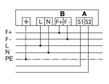
(A) Fail-safe contact. Series connection with other emergency lights. (B) Remote shutdown.
