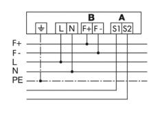
(A) Fail-safe contact.Series connection with other emergency lights.(B) Remote shutdown.
