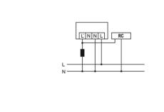
Standard operation parallel connection of max. 8 devices
