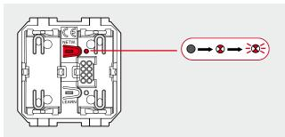
**3.** Press the NETWORK key on the interface. The NETWORK LED will come on steady during the network search procedure and then will start flashing slowly.
