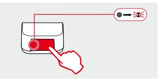
**2.** Press the NETWORK key again for at least 10 seconds. The NETWORK LED will flash quickly twice and then will turn off. The interface is no longer connected to the ZigBee network.
