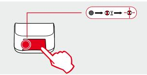
**4.** To complete the procedure press the NETWORK KEY of the Coordinator device; the corresponding NETWORK LED will flash three times while the interface NETWORK LED will turn off.
