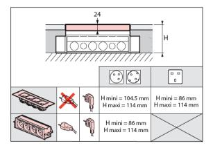
Box cross-section with height specification for horizontal support installation
