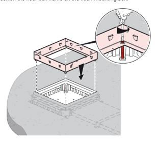
3) After laying the tiles, level the floor box frame with respect to the finished floor surface.
