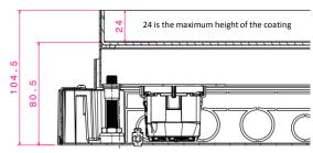
Min. concrete height 80.5 if coating (tiling + adhesive) = 24 mm If coating < 24 mm, concrete height = 80.5 + 24 - coating
