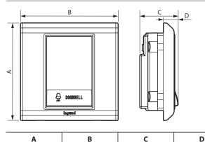
Distance of installation hole: 60.3 mm
