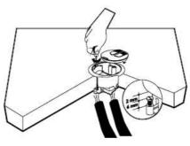
Fixing the floor boxes in concrete with plastic floor boxes ref 0 896  $49\,$
