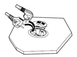
The support inside floor boxes 3 modules rocks and makes it possible to insert a side outlet plug & straight outlet plug
