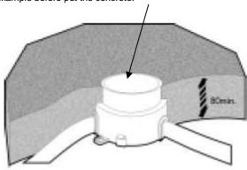
Technical floor is cut out according to floor boxes 3 modules:
