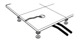
To carry out a % of turn of the screws inside the floor boxes to release the claws then to screw home (the claws are fixed under the technical floor)
