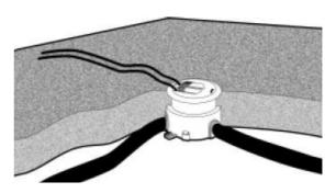
To carry out a % of turn of the screws inside the floor boxes to release the claws then to screw home (the claws are fixed under the edge inside the plastic floor boxes)
