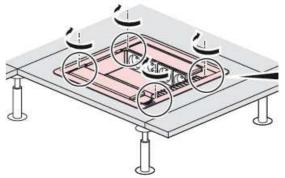
Technical floor is cut out according to dimensions below:
