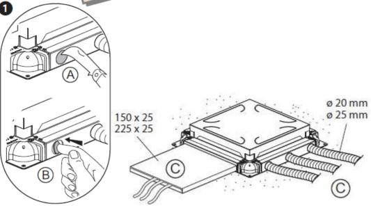
1- Put the trunking or flexible conduits (use a tool to fold), the side plates have to be cut out to fit the required ducting and/or conduits
