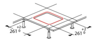
Dimension of the cover on the floor = 283x283mm
