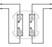
Type of terminals: with screws NO and/or NC contacts Terminal capacity: 1.5 mm<sup>2</sup> - 2.5 mm<sup>2</sup> (1 or 2 conductors) Stripping length: 12 mm Screwdriver: flat-blade 3.5 mm
