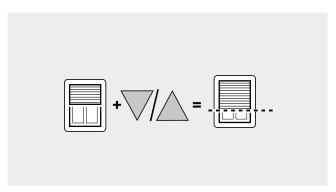
2. To save the desired position press the Preset pushbutton of the rolling shutter radio control for more than 10 seconds.
