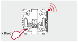
From now on, irrespective of its position, when the Preset pushbutton of the control device is pressed the rolling shutter will move to the previously saved position.
