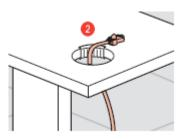
Put the cable between the dest grommet and the cable protection
