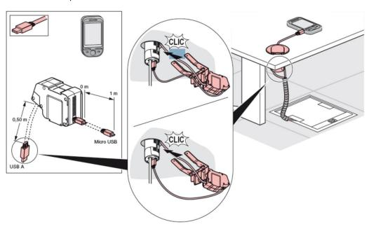
Installation with cellphone without retractable module USB/micro-USB
