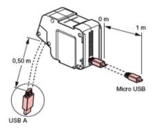
Cable 1.7x8mm in lenght of. 1m + plug USB micro B
