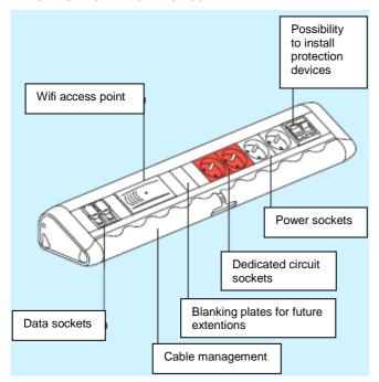
16A max (6A with filter) 3680W on 230V
