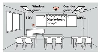
(\*) The **Display board** group is only possible if the installation includes a DALI unit Cat. No. 0 488 76. The lighting is only switched on when presence is detected and can be switched off with a push-button.
