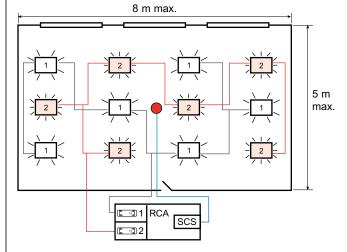
The 2 channels are synchronised. This enables the luminaires to be placed in staggered rows.
