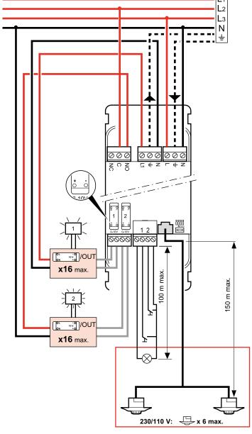
The two channels are synchronised, which enables the luminaires to be placed in staggered rows with one ballast supply phase on each channel.
