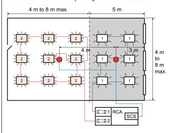
The BUS detector(s) are connected to the controller. In these modes, the controller applies a dimming difference of + 30% (mode 1), + 50% (mode 2) and + 80% (mode 3) between channel 1 (window side) and channel 2 (corridor side).
