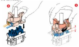
Spreading the wires ensures that pairs are separated by the required 13 mm.
