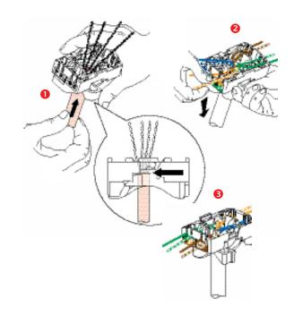
It therefore ensures the simultaneous connection of the cable strands.
