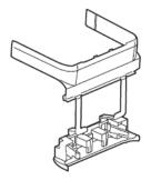
0 112 50: Derivation starting from a section width 105mm allows equipped with a cover 65mm towards a section width 105mm equipped with a cover 65mm
