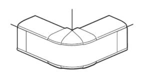
The junction in exterior angle of two pieces of the same section: - the cut of miter avoids on the trunking
