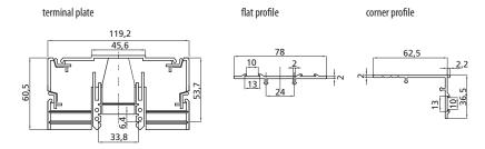
The covering UPO is the improved form for covering the space between rows of built-in elements in distribution boards. The built-in elements are installed on the mounting rails with width of 35 mm which shall be mounted in the distance of 125 mm.
